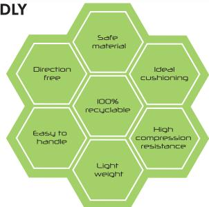
Eltete honeycomb board is a 100% recyclable carton product. Its hexagonal structure provides extraordinary strength, and makes it suitable as protection for transport packaging and also for a multitude of other applications.
