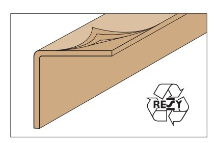
Raw Material. The standard edgeboard is manufactured by laminating several layers of strong paperboard.
