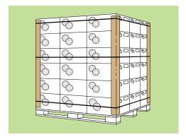
Edgeboards stabilise the pallets and provide protection during transport and warehousing.
