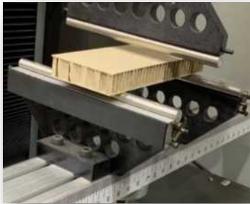
Bending Strength Test for Honeycomb Board
