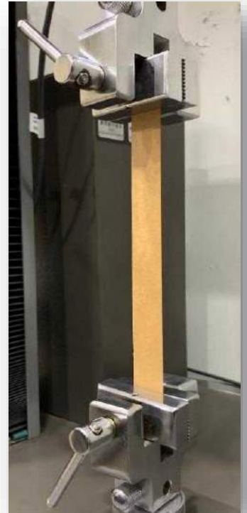
Tensile Strength Test for paper & Slip Sheet
